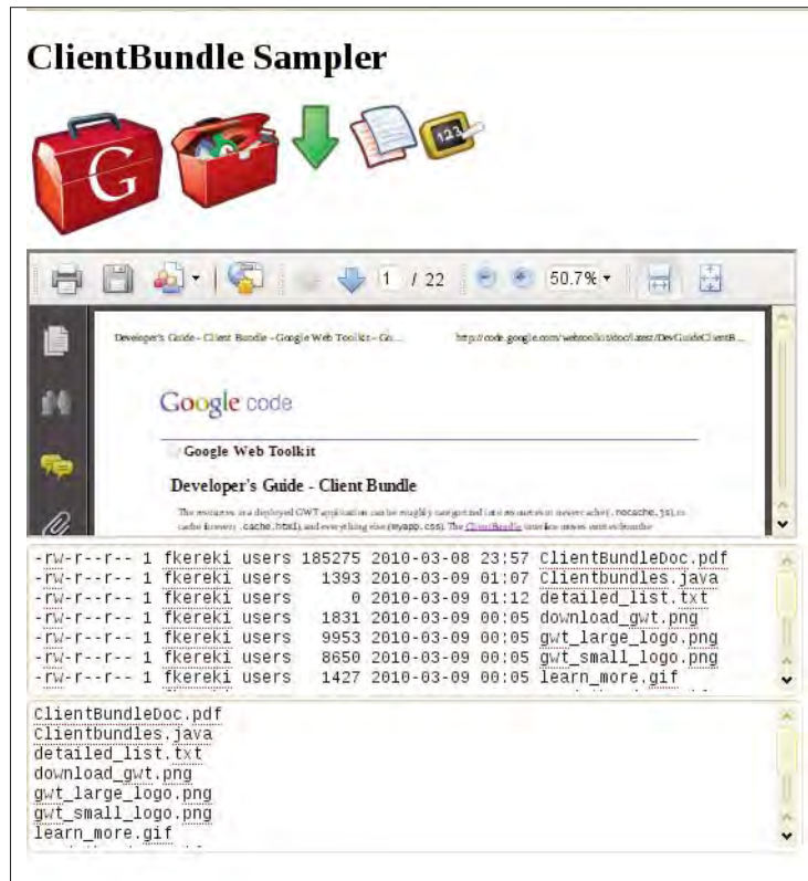
Figure 14.2 A sampler application, showing the usage of resource bundles to display some images, a PDF file, and text files by two different means.
