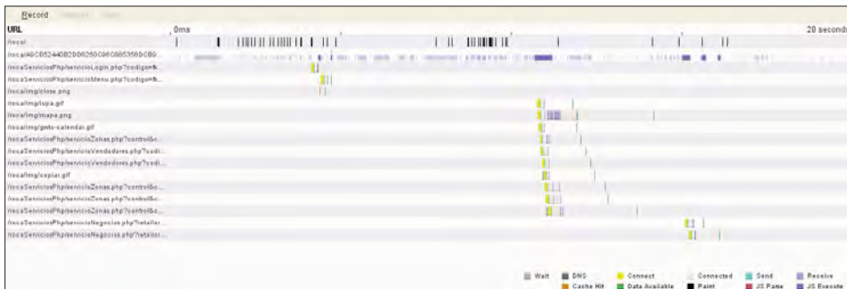
Figure 14.12 The Page Speed Activity lets you analyze a timeline for your application, detecting bottlenecks and too many concurrent calls.
